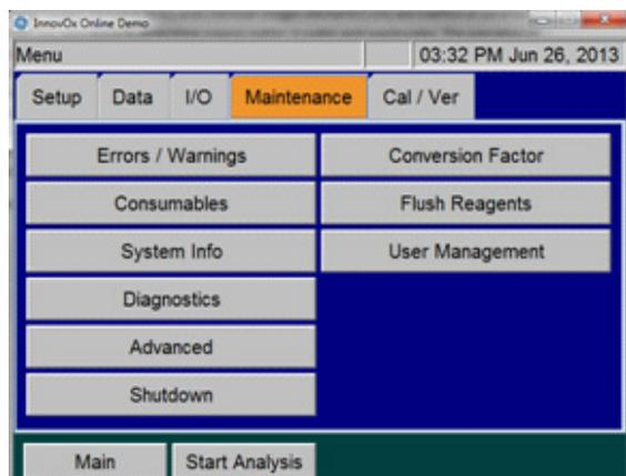
Figure 2. InnovOx Analyzer operation screen showing where to locate the conversion factor option.
