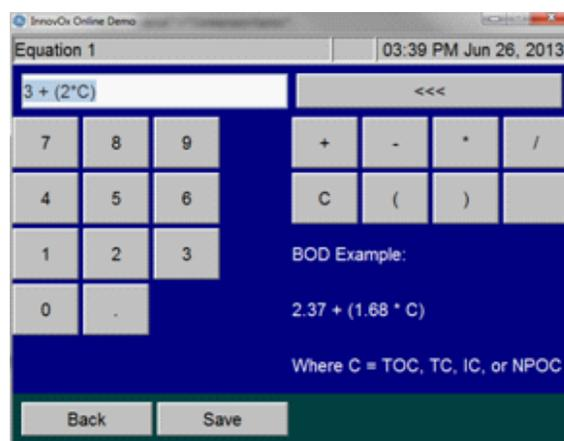
Figure 3. InnovOx Analyzer operation screen showing where to enter the conversion factor.
