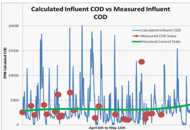
**Figure 1.** InnovOx Analyzer data and the actual COD measurement comparison chart.
